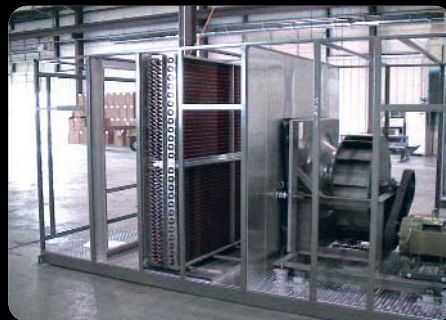
Conventional air handler fan section
