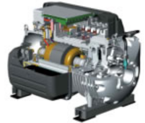
Turboacor compressor features oil-free design, single moving part, magnetic bearings.
